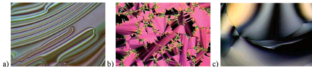
FIGURE 5. Textures of 6'- n -decyl-6-(5- n -undecylthiophen-2-yl)[3,3']bipyridinyl 26b observed by optical microscopy (a: 138.4 °C, SmC (freely suspended film); b: 122.9 °C, SmF (slide); c: 125.4 °C, SmF (freely suspended film).
